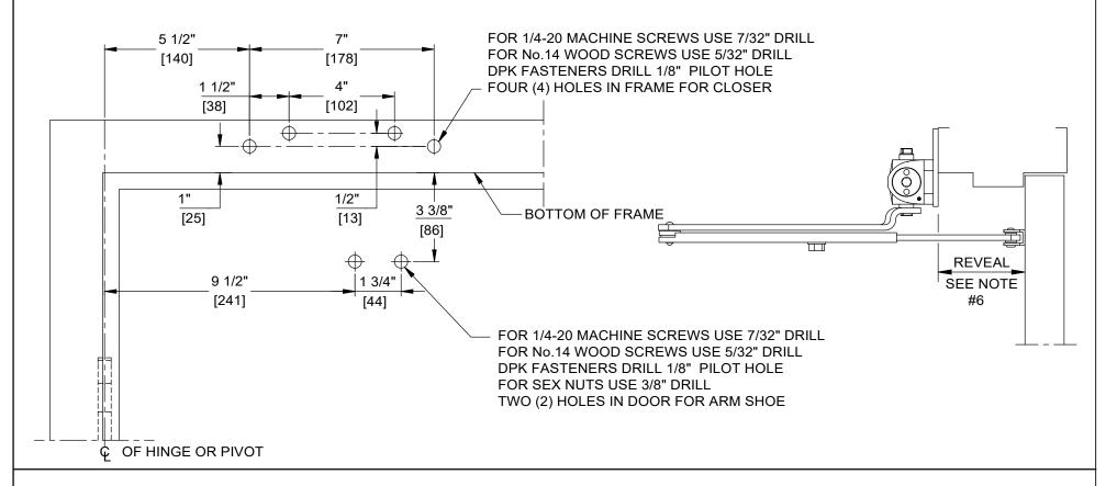
DOOR CLOSER MODELS: 8616 AFJ OR ARJ (NHO) TOP JAMB INSTALLATION (PUSH SIDE MOUNT) WITH PLATE DP86
