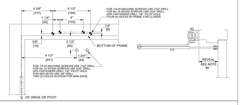
DOOR CLOSER MODELS: 8616 AFJ OR ARJ (NHO) TOP JAMB INSTALLATION (PUSH SIDE MOUNT) WITH PLATES BP86, BP86FC
